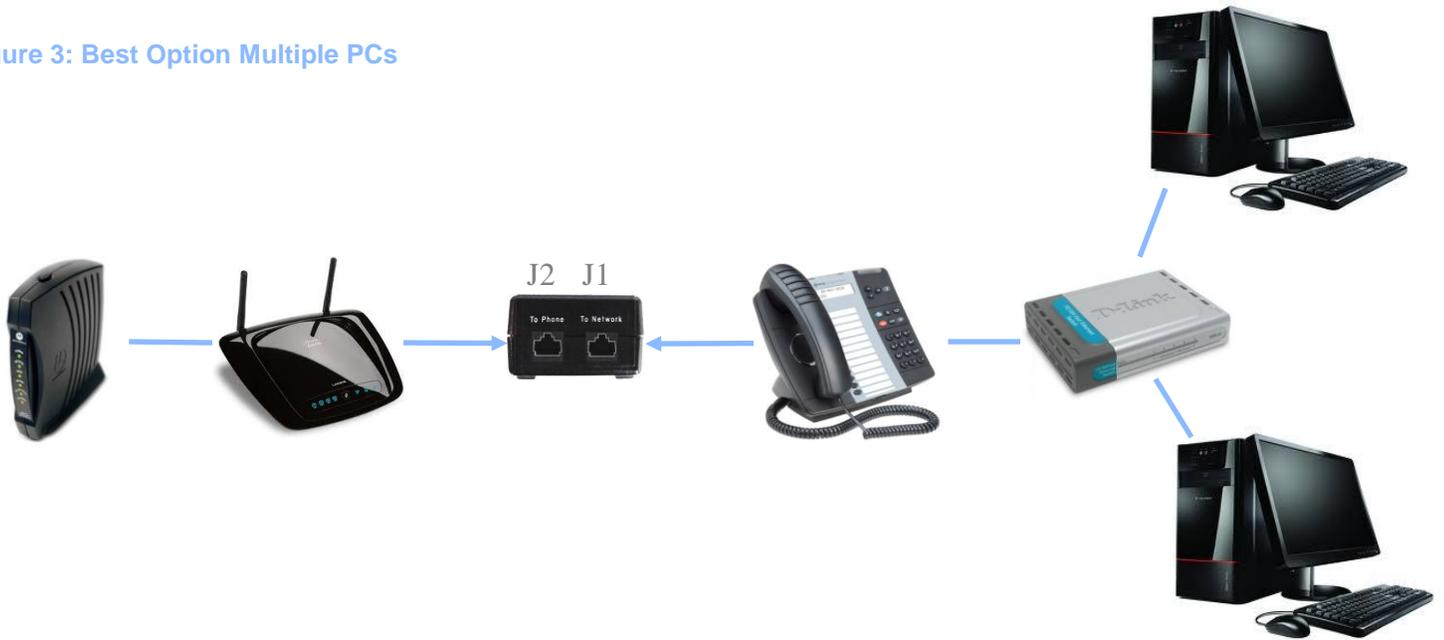
When there are multiple PCs on the home LAN, the optimal configuration is to have the phone connected directly into the router, and a switch connected into the PC port in the phone. This will allow multiple PCs to connect via the switch, and still allow the phone to prioritize voice IP traffic over other traffic.
